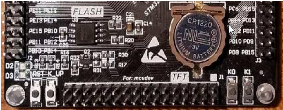
FSMC LCD Connector – Top View (Old – TFT0)
